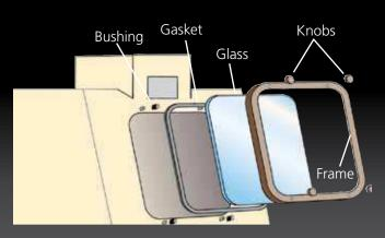
**Safety-Glass Window** (14"x 22") provides large viewing area, can be changed in a few minutes without tools and has rounded corners for safe handling.
